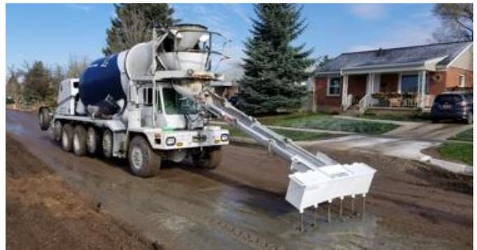
Fig. 2. Front-discharge truck with an attached Slurry Spreader.
