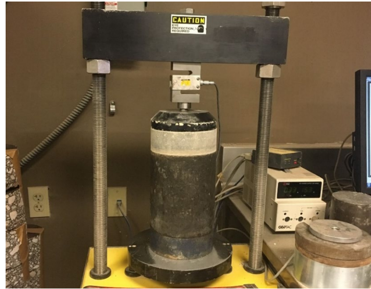
Unconfined compressive strength test
